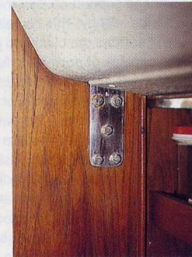
Offset shroud load on the chainplate can cause moisture to get into boltholes, swelling the bulkhead
