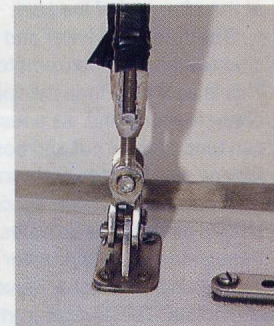
Chainplates for the lowers and cap shroud are small. The clevis pin can draw out or shear its locking pin
