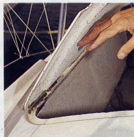
Locker lids are foam-cored for stiffening, but have been known to delaminate
